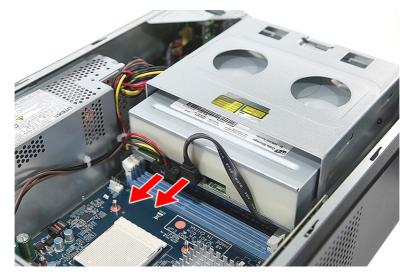
(2). Remove the two screws (B) that secure the HDD-ODD bracket.
